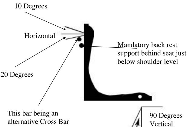
alternative Cross Bar behind the Seat, applicable when the seat belt is taken over and downwards
